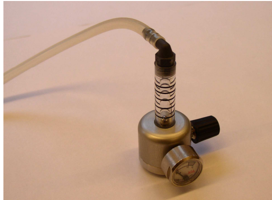
Valve with flowmeter fits the Geopal test gas cans.
